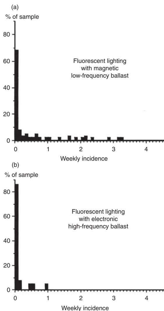
**Fig. 2.** Percentage of a sample of office workers experiencing different frequencies of headaches per week, while working under fluorescent lighting operated on magnetic (50 Hz) control gear and electronic (32 kHz) control gear (after 23).
