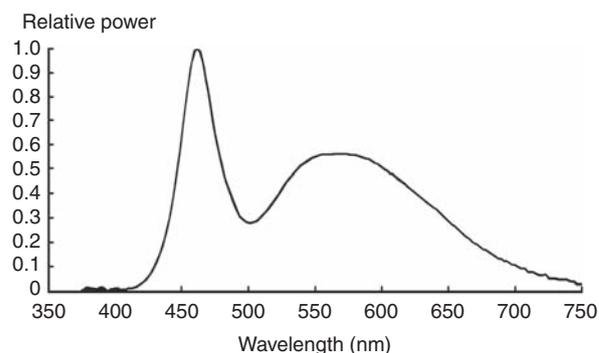
**Fig. 1.** The relative spectral power distribution of a white LED. This is basically a blue LED with an integral phosphor.
